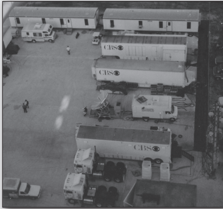
Figure 1.5 1985 Daytona 500 CBS mobile units MU8a and MU8b plus a support trailer that carries cable and additional equipment and has a complete maintenance area.
